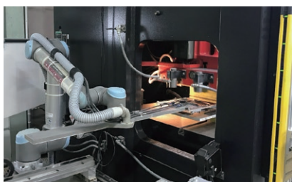
社内運用プレス加工自動供給ロボット Automatic supply robot in in-house operation for pressing process
