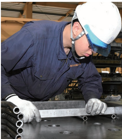
パイプの両端の幅を測り、寸法を確認 Dimensional check by measuring the width of both ends of a pipe
