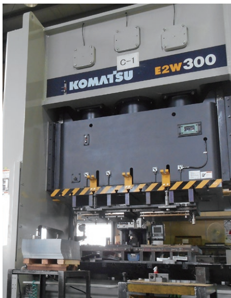
当社保有の最大加圧能力の300tプレス機 Our greatest pressing machine able to exert up to 300 t
