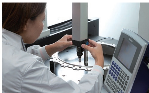
三次元測定機による検査風景 Testing with a three-dimensional measuring machine
